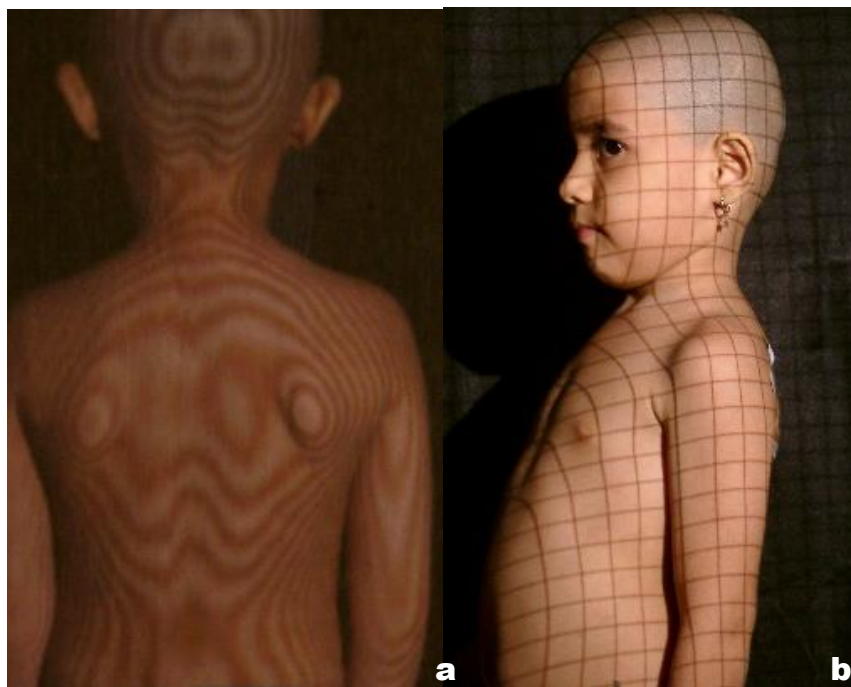
Fig. 1. (a) Study of human back using moiré fringe topography and (b) human shoulder using rasterstereography
