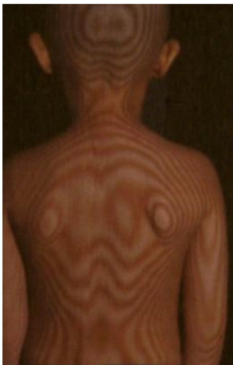
Figure 1. Study of human back using moiré fringe topography (Credit: Shakeel Ahmed Ansari)
