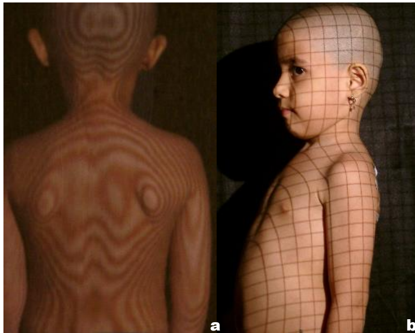
Fig. 1a, b. Studies of (a) human back using moiré fringe topography (photo credit: Shakeel Ahmed Ansari) and (b) human shoulder using rasterstereography (photo credit: Majeed Ahmed Khan)
