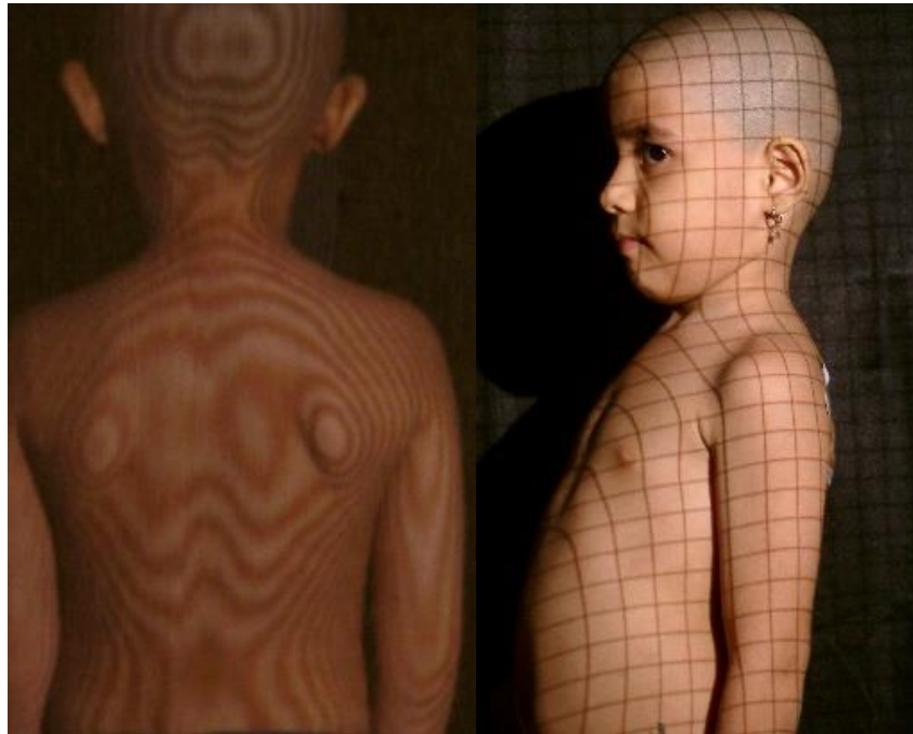
From left to right, studies of human back using moiré fringe topography (photo credit: Shakeel Ahmed Ansari) and human shoulder using rasterstereography (photo credit: Majeed Ahmed Khan)
