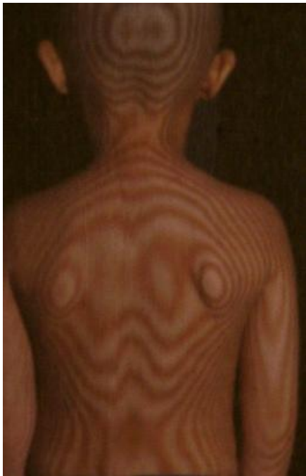
Figure 1. Study of human back using moiré fringe topography (Photo Credit: Shakeel Ahmed Ansari)
