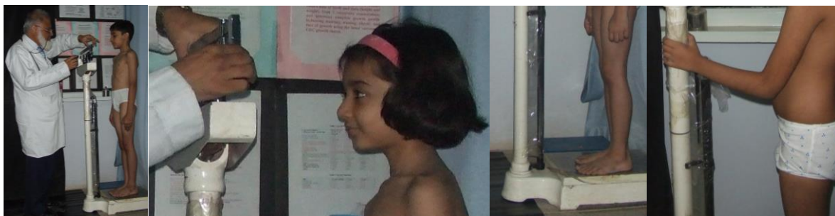
Fig. 1. From left to right, (a) measurement of mass; common errors in measurement process (b) hair-band not removed; (c) feet not positioned correctly and (d) student holding on to beam scale
