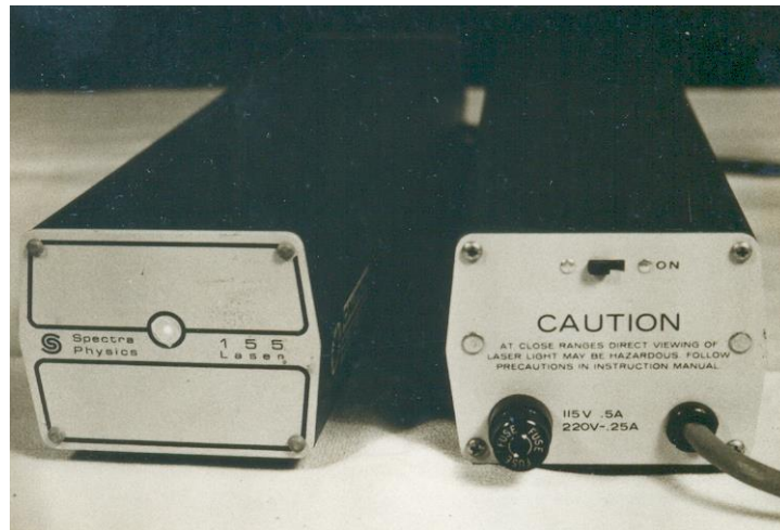
FIGURE 2: Laser beam type 155 used in this study.
