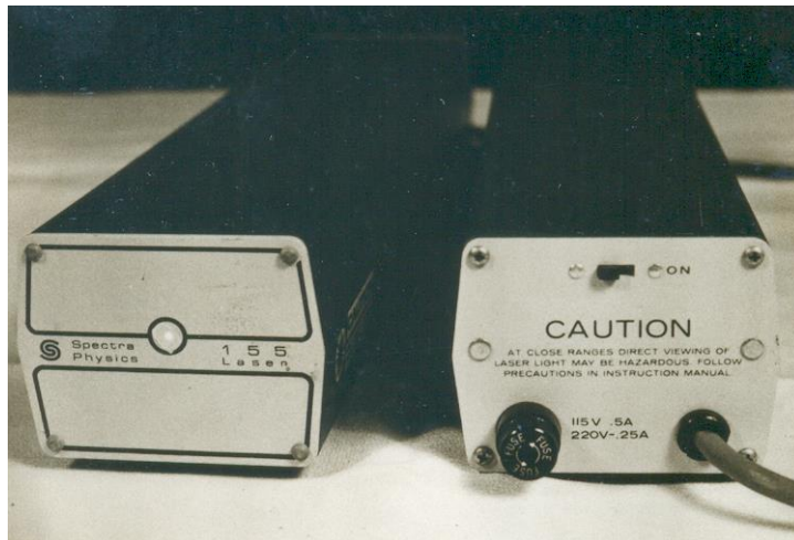
Fig. 2. Laser beam type 155 used in this study
